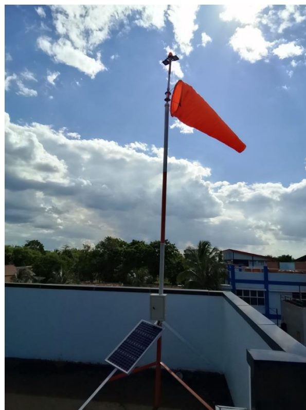
Figure 4. Test of Portable wind direction indicator
