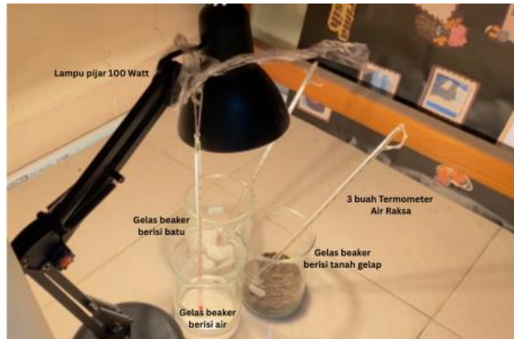
Figure 1. Experimental setup for radiation and albedo
