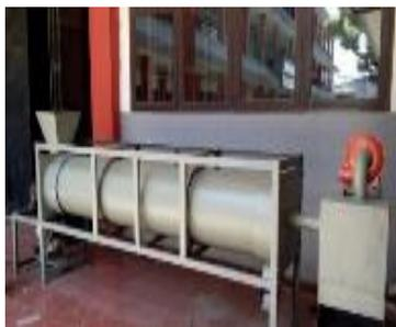
Gambar 4. Pengering Gabah Sistem Rotary Dryer
