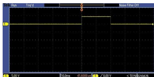
Gambar 13. Hasil Time Period PWM saat suhu 30-40°C
