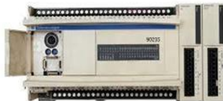
Gambar 2. PLC schneider twido [2]-[4]
