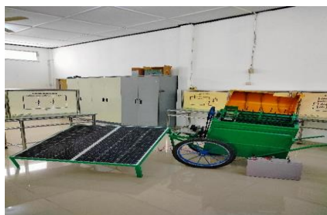
Gambar 3. Power thresher solar cell
