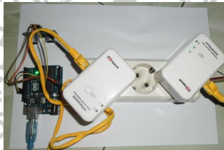
Gambar 7. Foto Rangkaian Sensor Ultrasonic Arduino melalui Komunikasi Modem Power Line Communications
