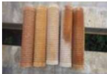
Gambar 1. Microfilter Cartridge Bekas sebelum Chemical Cleaning Citric Acid
