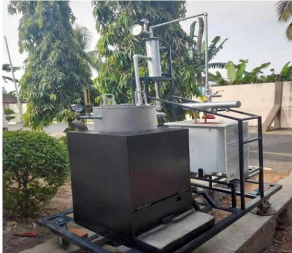
**Gambar 1.** Unit *Thermal Cracking Reactor*
