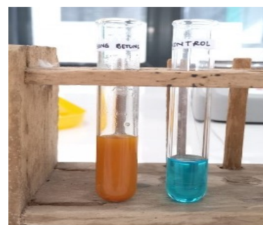
Figure 1. Benedict's test results on bamboo shoot flour (orange in color) and negative control benedict's test (blue in color)
