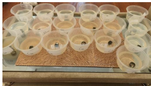
Figure 3. Carbon steel pipe immersion
