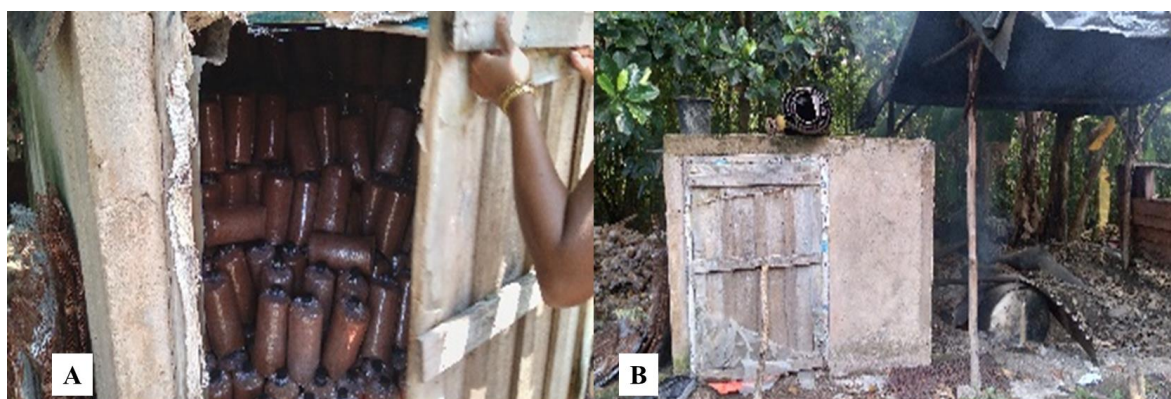
Figure 2. Pasteurization equipment. A. Transferring the baglog into the pasteurization equipment, B. Pasteurization process.
